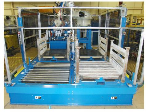
Once the stack layer has been achieved, the robot will place a slip sheet on the pallet or rack until it is full.
