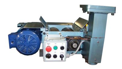
The MAC Paste Prep System mounts to the base of the cone feeder which mounts on a pivot so it can be rotated out from over the hopper for accessing the hopper, rotating the hopper up and for clean-up.
