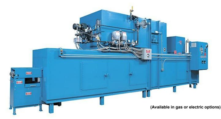
The **optaMAC Oven with an extended heated section** features 100% convection heat with a 304" (7722 mm) heated section and an overall length of 342" (8691mm). This oven is designed for customers using high speed continuous lines.
