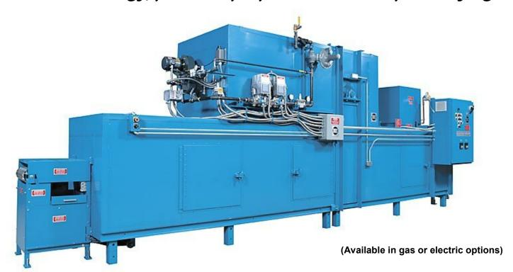
The optaMAC Oven with an extended heated section features 100% convection heat with a 277" (7036 mm) heated section and an overall length of 319" (8102 mm). This oven is designed for customers using high speed continuous lines.
