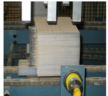
Picture 2: Precision aligned stacks after Stack Aligner
