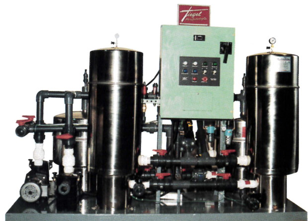
Tiegel's Wash Maximizer I recirculates the wash water through its unique acid-sponge beds, filtering out impurities and recycling 99 percent of the acid.
